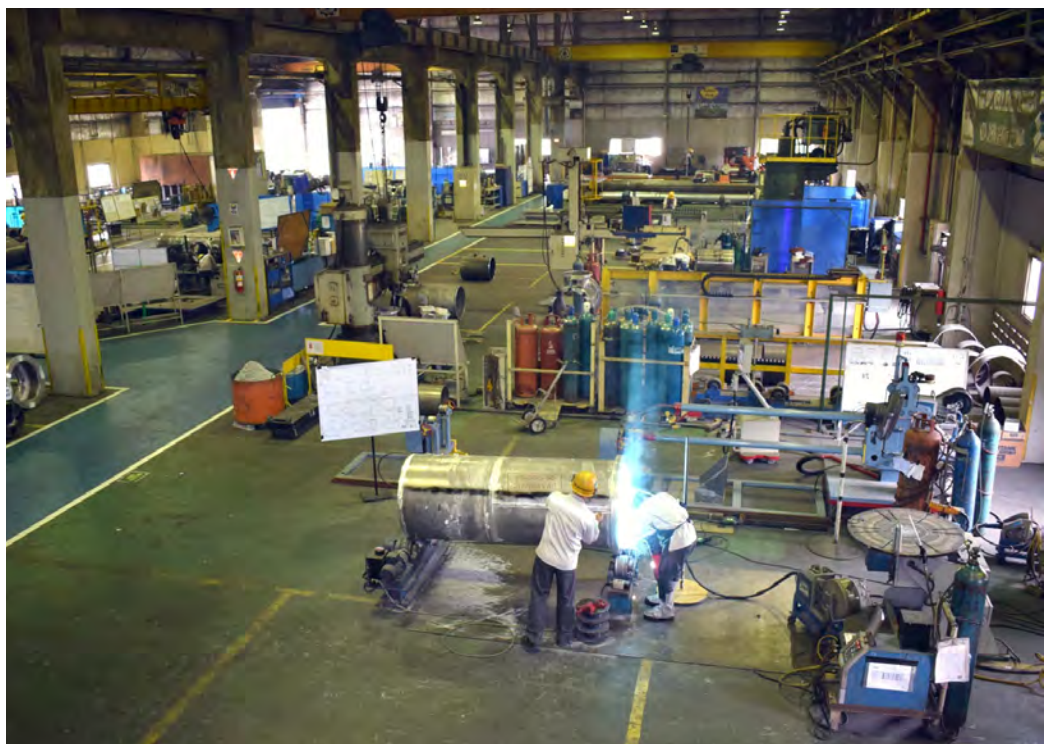
Part of the fabrication shop where the enclosure of the GIS called GIS Tanks and conductors are fabricated.
