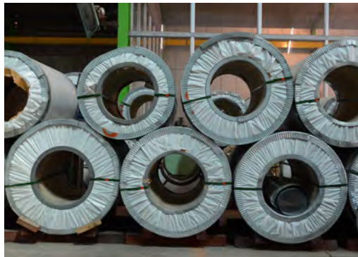
Grain Orientated Silicon Steel Core
