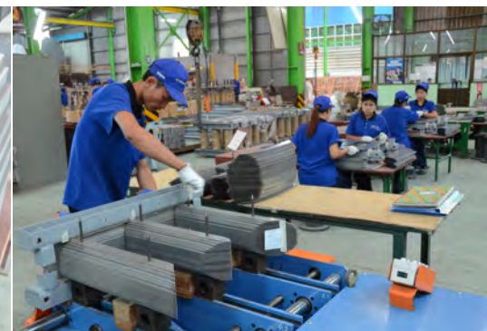
Production of the stacked magnetic core
