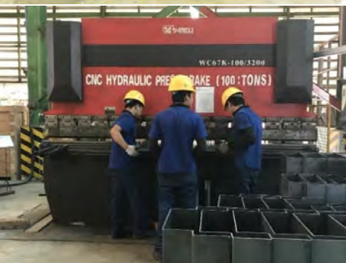
Production of Transformer Tank body by CNC Plasma Cutting Machine & CNC Pressbrake
