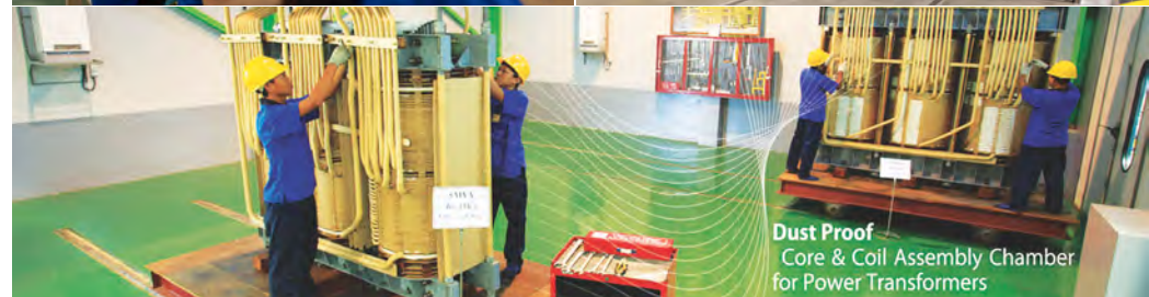
Core and coil assembly at different stages of the transformer
